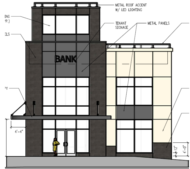
The design of Building 2, as shown by elevation facing City Avenue, includes a tower feature to accentuate the site's importance as a gateway site.
