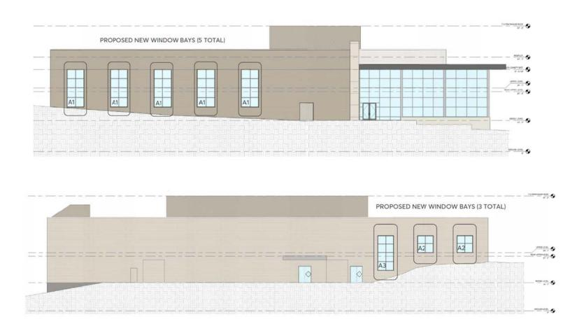
Revised Front and Side Elevations with 8 (total) New Window Openings
